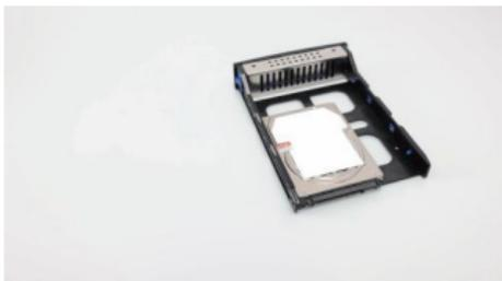
For 2.5"SSD/HDD: Use screwdriver open the blue clasp on the side.
