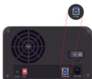
Connect the USB 3.0 connector to the unit
